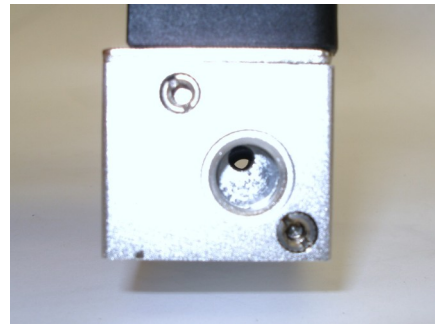
Figure 3: Default inlet/outlets on the side of the assembly.
